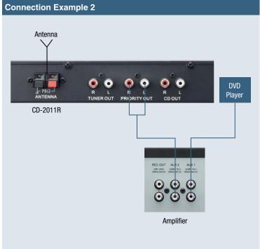
When there is a limitation in AUX input, Priority Out terminal can be connected so that the output for CD mode and Tuner mode is combined, but in the following priority: CD, USB, SD/MMC Card, FM Radio.
