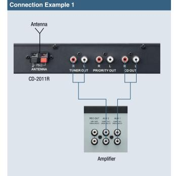
With this connection, Tuner mode and CD mode outputs can be controlled separately.
